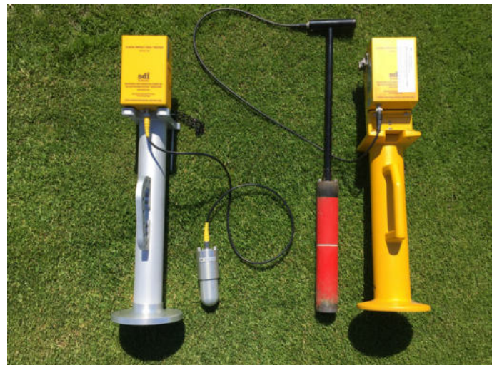
Indirekte Messung: Clegg Impact Soil Tester (CIST) = Clegg Hammer
