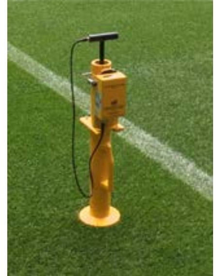
Abb. 9: Clegghammer (Clegg Impact Soil Tester). (Foto: H. Nonn)
