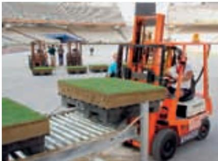
Photo 15: A forklift receives the module from the end of the roller conveyor line and transports it to its final position.
