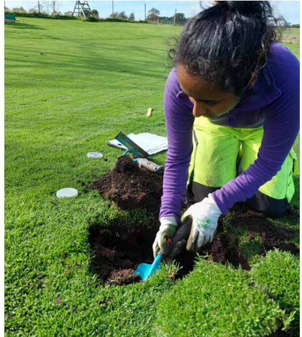
Monica Jayesingha taking undisturbed soil samples for soil density analysis at Berheim GC in September 2023. Photo: Anne F. Borchert.
