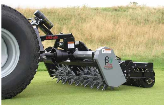
Picture 18. The Aeravator is popular for ice cracking because it is robust and flexible. The rolling tines vibrate. Efficient, but the risk of damaging the green is high.
