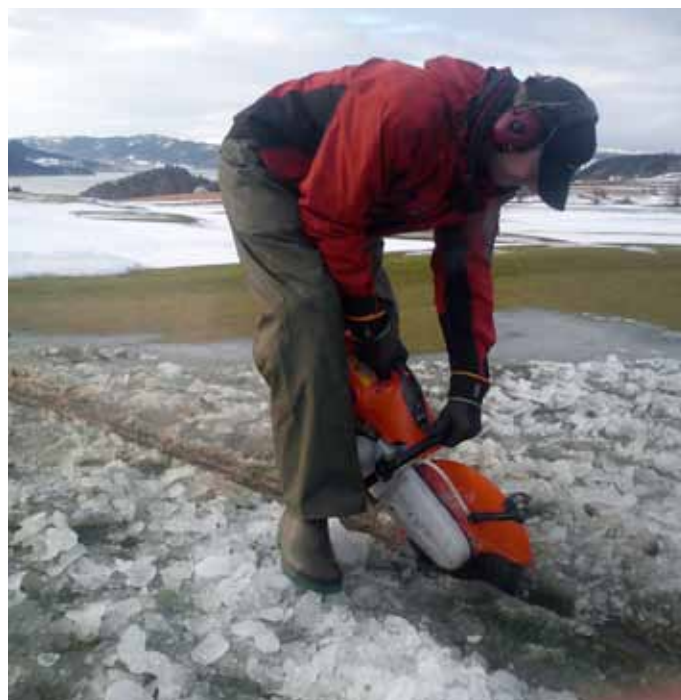
Picture 13. Temporary ditches in greens need maintenance during the winter. An asphalt cutter is used at Byneset GC, Norway. Photo: O.A. Kjøsnes.
